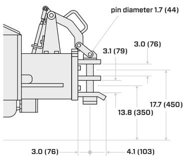
PIN TYPE DOUBLE STAGE DRAWBAR<sup>2</sup>
